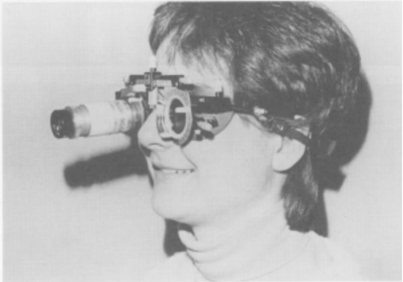
*Figure 3.* Subject wearing trial frames and blurscope to restrict resolution.
